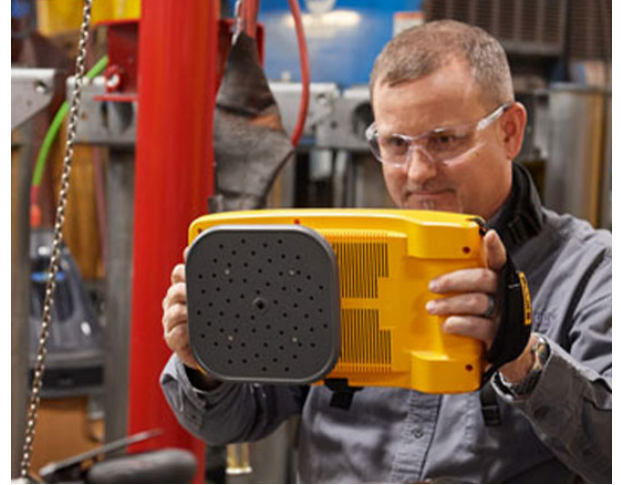
Figure 4: Detecting leaks using the full array microphones.
