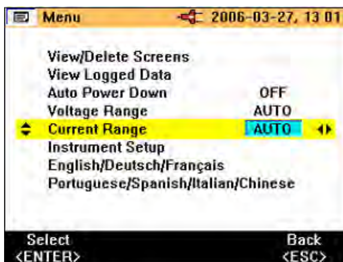
Figure 13. Current Range Settings
