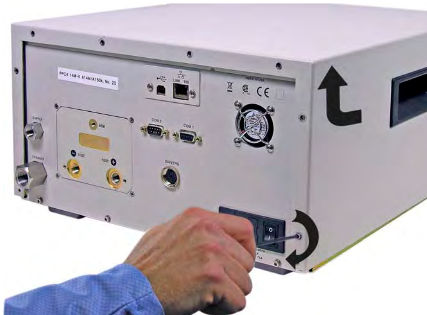
Figure 15. Removing Back Cover
