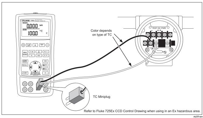
Figure 16. Connections for Simulating a Thermocouple
