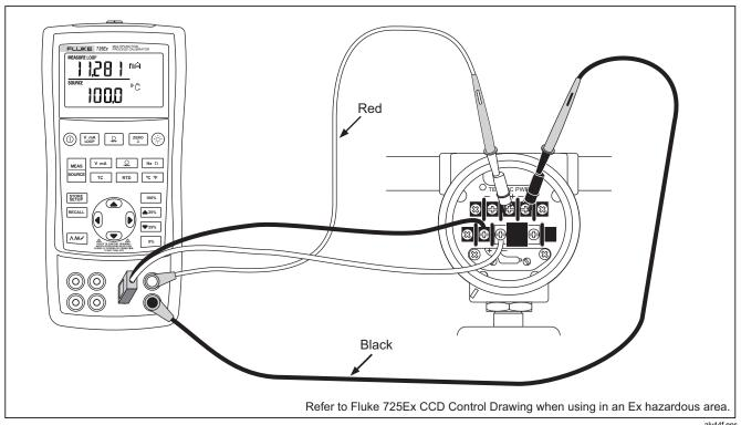
Figure 19. Calibrating a Thermocouple Transmitter
