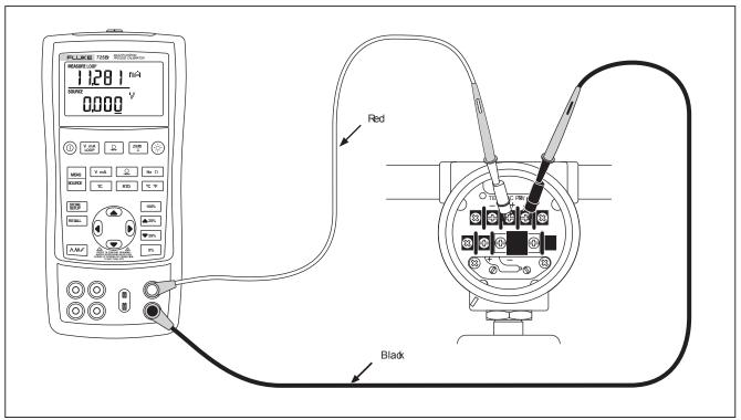
Figure 8. Connections for Supplying Loop Power
