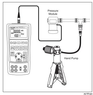
Figure 18. Connections for Sourcing Pressure
