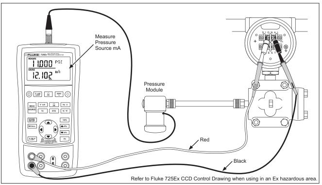
Figure 21. Calibrating a Current-to-Pressure (I/P) Transmitter
