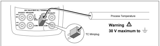
Figure 10. Measuring Temperature with a Thermocouple
