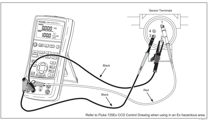
Figure 17. Connections for Simulating 3-Wire RTD
