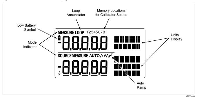
Figure 4. Elements of a Typical Display
