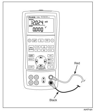
Figure 7. Measuring Voltage and Current Output
