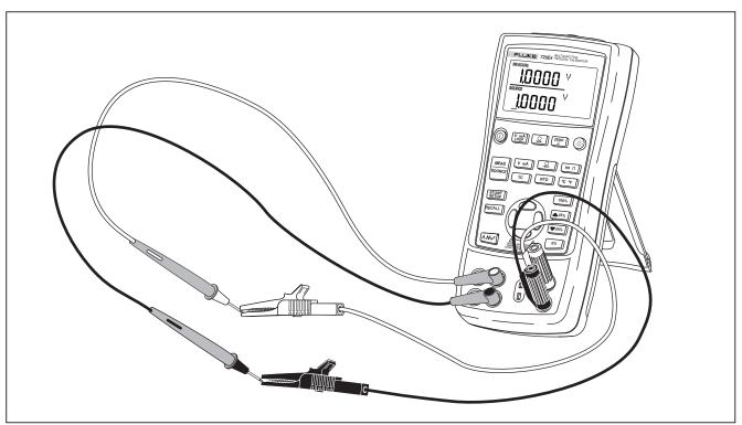
Figure 5. Voltage-to-Voltage Test
