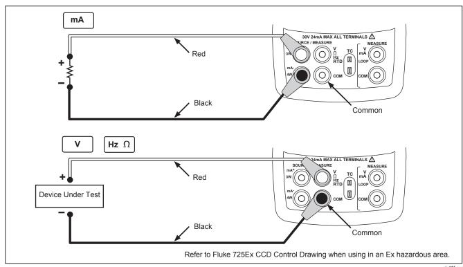
**Figure 15. Electrical Sourcing Connections**
