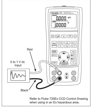
Figure 22. Calibrating a Chart Recorder
