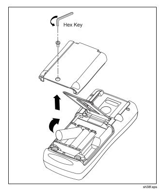
Figure 23. Replacing the Batteries
