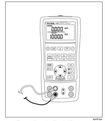
Figure 9. Measuring Electrical Parameters
