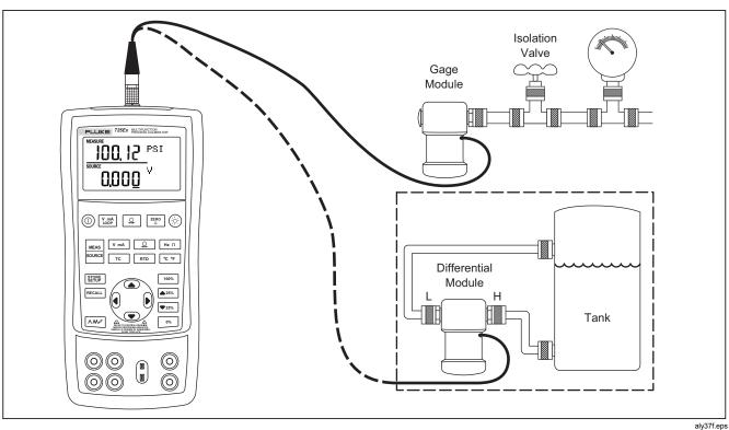
Figure 13. Connections for Measuring Pressure
