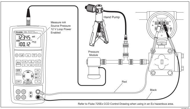
Figure 20. Calibrating a Pressure-to-Current (P/I) Transmitter
