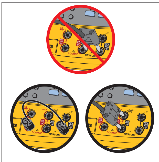
Figure 16. Correct Jumper Use
